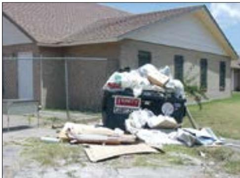
The photo on the left shows a trash dumpster that is overflowing and too close to the building. If vandals were to intentionally set fire to the dumpster, there is a high likelihood that it would spread to the building.
